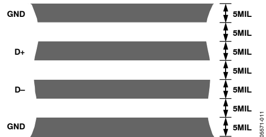
Figure 23. Typical Arrangement of Signal Tracks
